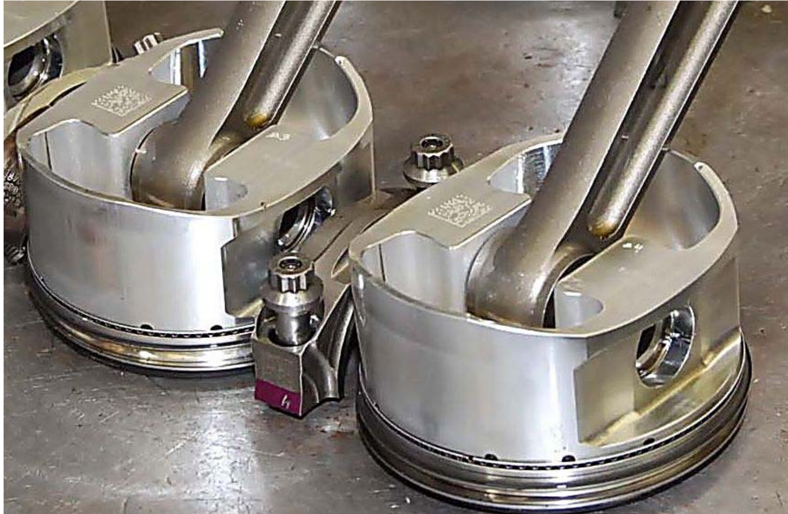
LS2 JE Piston Skirt Wear 1000 Miles - Racing.
