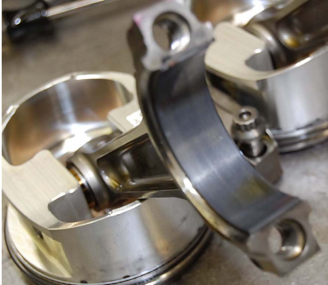
LS2 Rod Bearing Wear 1000 Miles - Racing.
