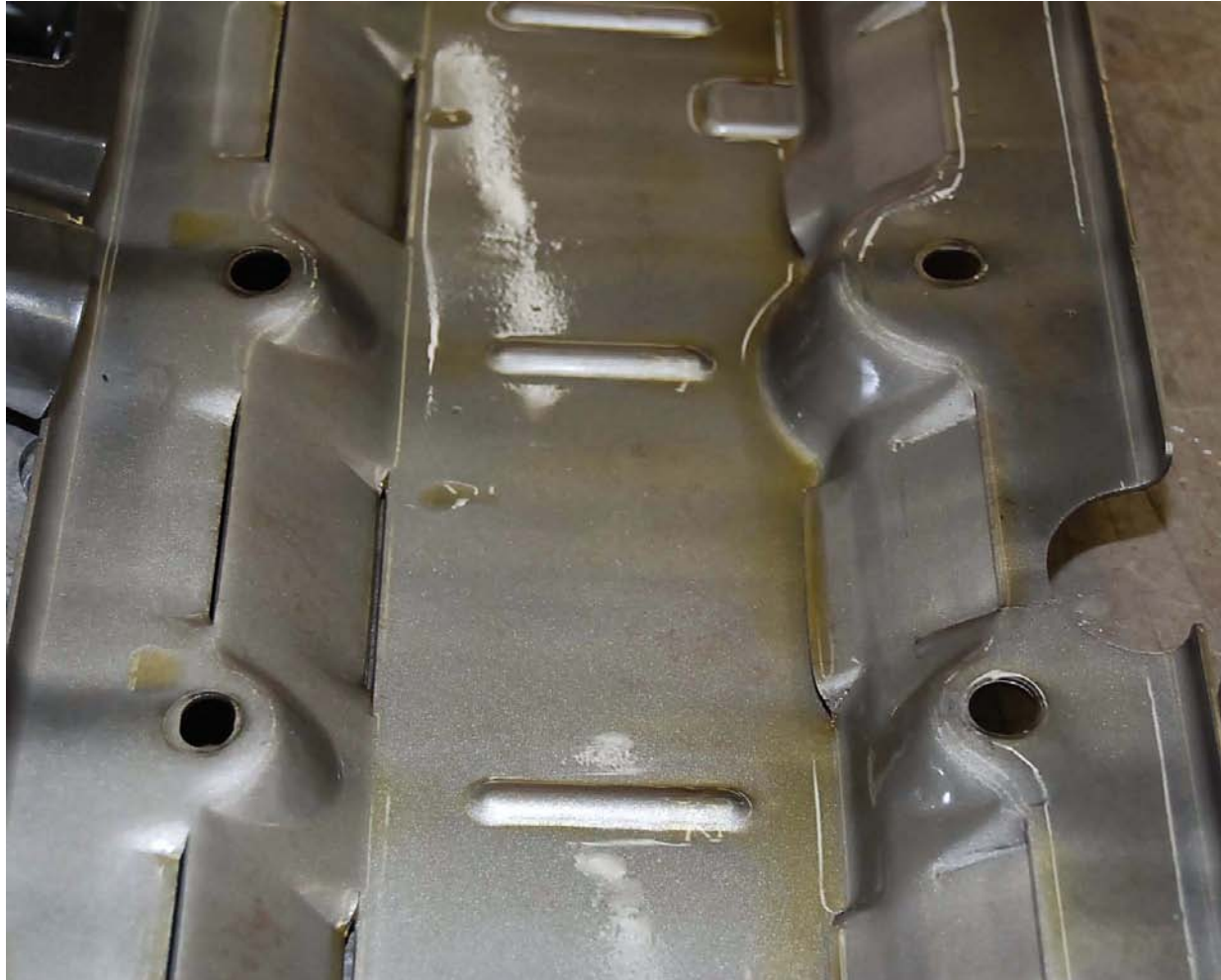
LS2 Motor / Pan Cleanliness 1000 Miles - Racing.
